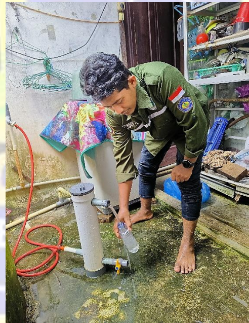
Gambar C.6 Pengujian Unit Pre-treatment Titik Sampling I
