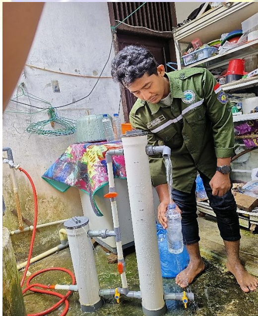
Gambar C.5 Pengujian Unit Filter dan Unit Pre-treatment Titik Sampling I
