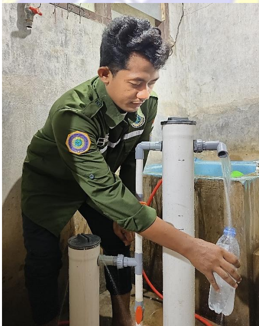
Gambar C.8 Pengujian Unit Filter dan Unit Pre-treatment Titik Sampling II
