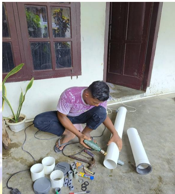
Gambar B.3 Perakitan Filter
